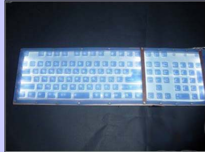
Flexible Rubber keypad with plastic keycaps , powered through a standard USB cable.
