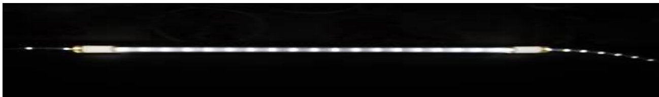
Figure 7 HOW – DOPI – DOPE system configured for signage channel letter has drastically reduced cost and makes for the first time a use of LEDs affordable also for large scale signage applications. Miniature DOPI Light Engines with few high efficacy LEDs and flexible fiber with directional point-like DOPE light extractors.
