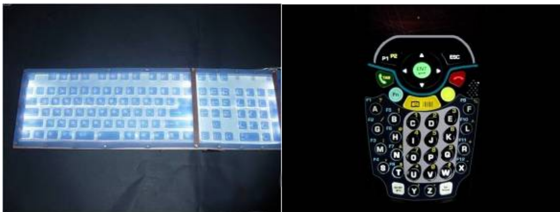
Figure 6. Ultra-thin HOW™ Keypad & Keyboard backlights feature up to x50 power efficiency compared to standard systems and use just one low-grade LED replacing 10-20 similar lamps. With a thickness of 100 – 200 um it is suitable for the slimmest MP and large keyboards.
